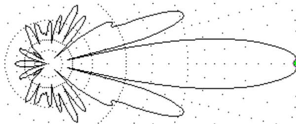
Pic.: Elevation Plot - 15 elem. LFA bay (G0KSC) over stacked by 0.4 m
