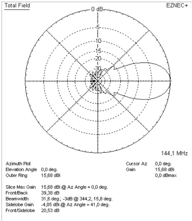
Azimuth Plot of a GTV 2-12n
