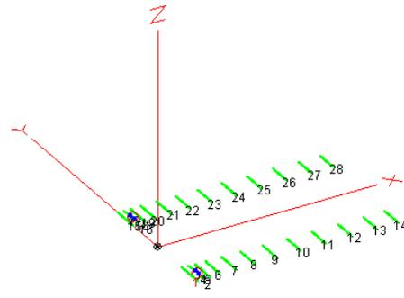
**Step 3:** Following that we lower the 2 Yagis by half the H-stacking distance of  $-(3,558 \text{ mm} / 2) = -1,779$  mm by using 'Move Wires XYZ' in Z-direction.
