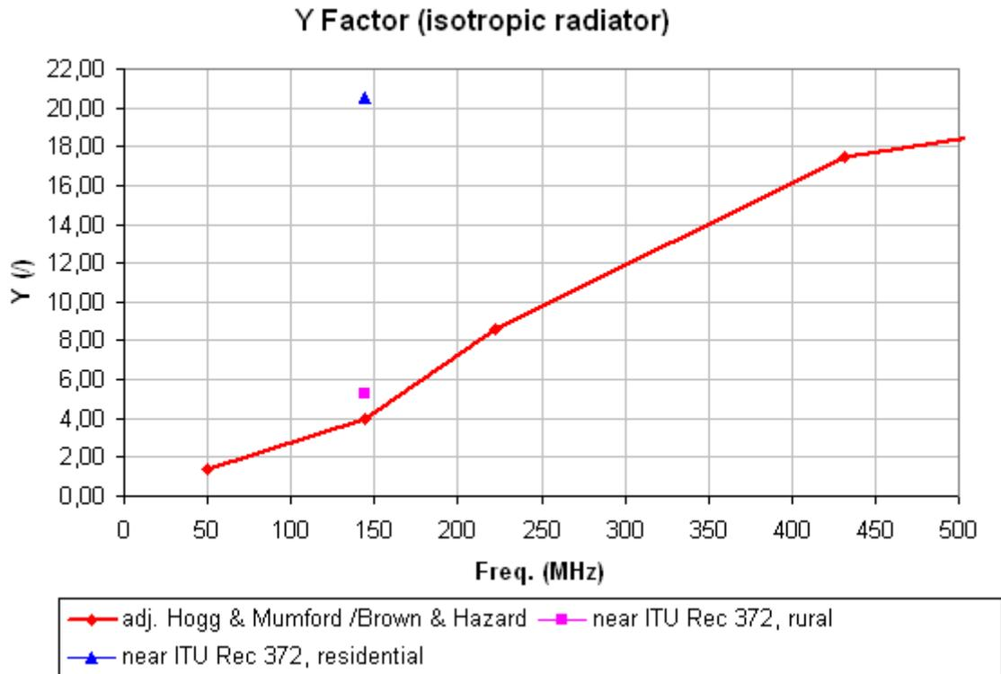
The chart indicates that caring for the G/T - ratio at the antenna fed point is approximately 3 times more important on 144 MHz than on 50 MHz and 9 times on 432 MHz. However newer findings for man-made-noise on VHF in accordance with the ITU recommendations [2] issued 2016 shows a Tearth as man-made-noise of 1308 K for rural areas and 5127 K for residential areas. Which highlights the importance of Antenna G/T on 144 MHz in such environments.
