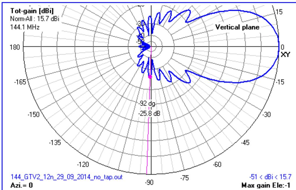
1. Click somewhere near to the suspected lowest F/R in the rear half of the plot and tick towards the maximum from -90 to +90 degrees using the left/right arrow keys.
