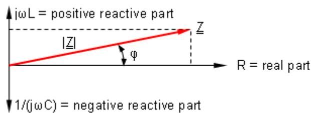
The G/T tables use 50.150 MHz / 144.100 MHz / 432.100 MHz as the target frequencies throughout, so we place the marker there and read out the complex impedance  $\underline{Z}$  [Ohm]. In our example (GTV 2-12n) we read  $\underline{Z} = (48.11 + j 0.14)$  Ohm or in Euler's notation 48.11Ohm at 0.17 deg. as the apparent impedance  $|\underline{Z}|$  from the data displayed in the EZNEC VSWR plot window:
