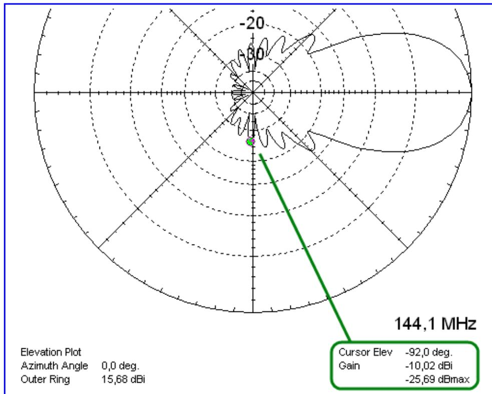
For the GTV 2-12n the F/R is close to the threshold of the rear half of the plot circle. We find an F/R ratio in compliance to the G/T Tables (-)25.69 dB at 92 degrees for this design. If we calculate this we get 15,68 dB - (-10,02 dB) = 25.70 dB.
