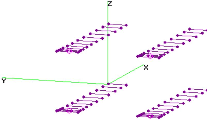
For a visual inspection of the stacking distances and proportions the 'Geometry' Window (F3 - key) is more suitable and displays without distortion.
