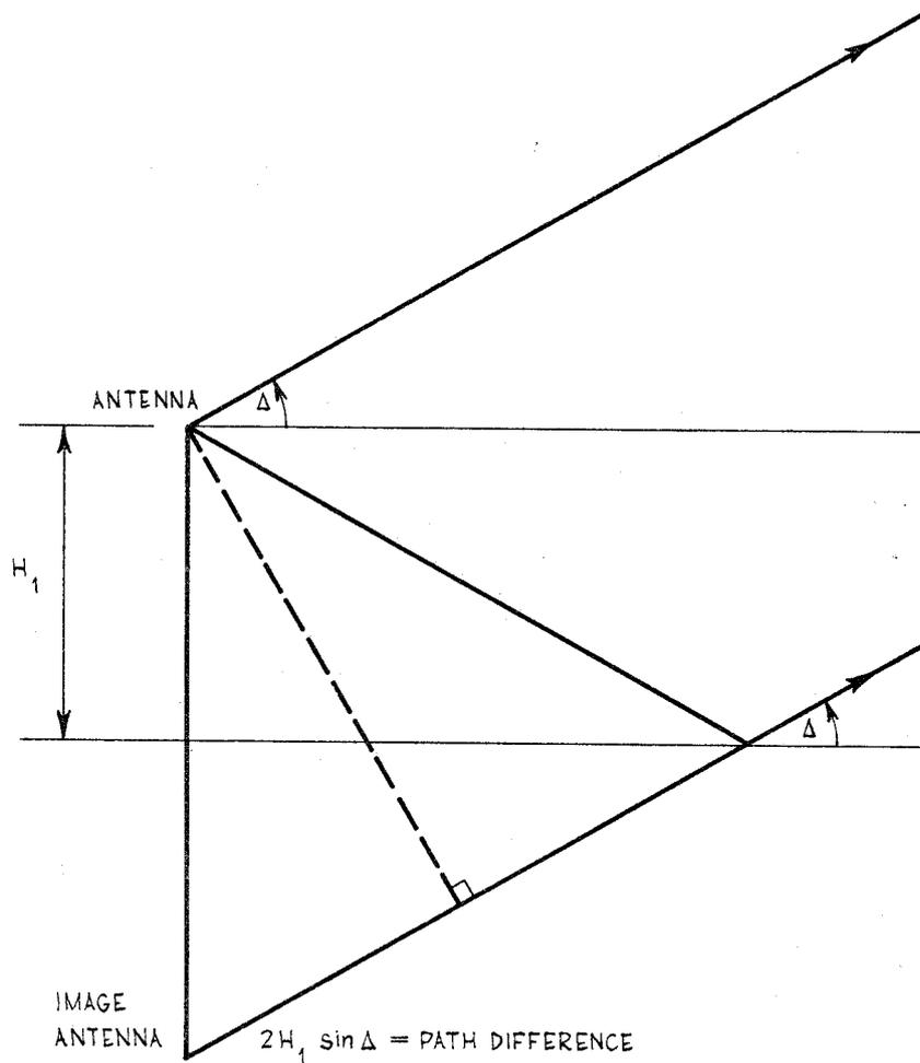
Figure 12. Geometry for Antenna Polar Diagram
