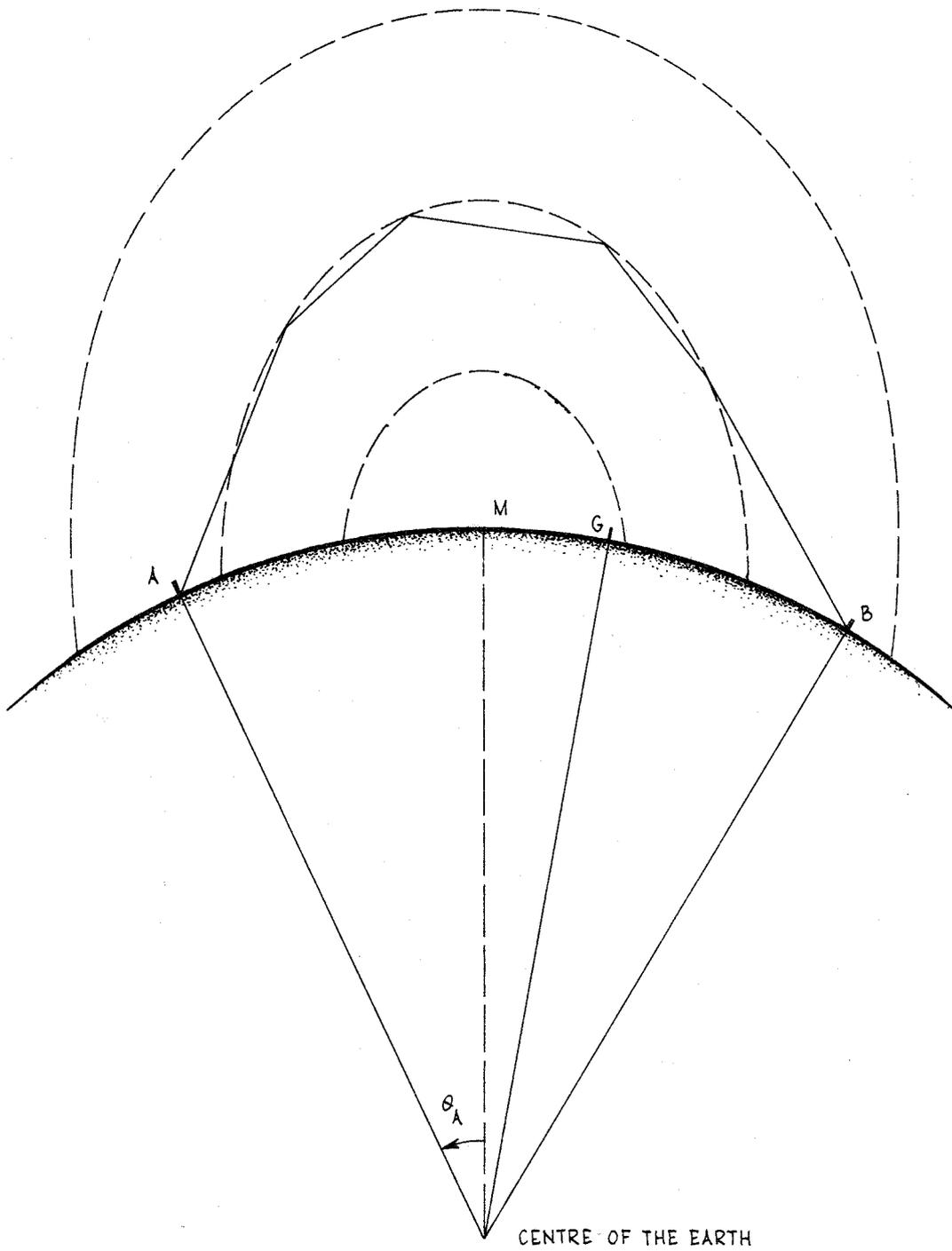
Figure 1. Power from a transmitter at A in one hemisphere is received at B on the opposite side of the geomagnetic equator
