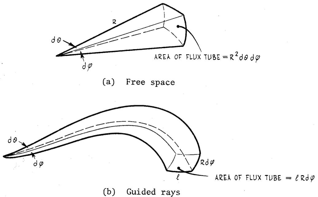
Figure 3. Illustration of the construction of flux tubes in (a) free space, (b) where guidance is involved
