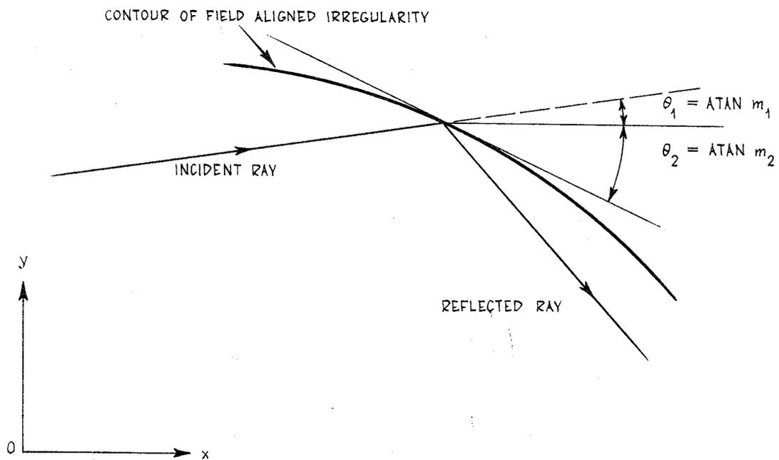
Figure 13. Geometry for reflection of a ray from an elliptic surface
